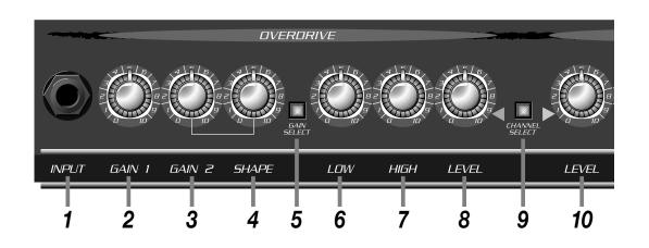
**1: INPUT:** Connect your guitar here using a shielded instrument cable.
